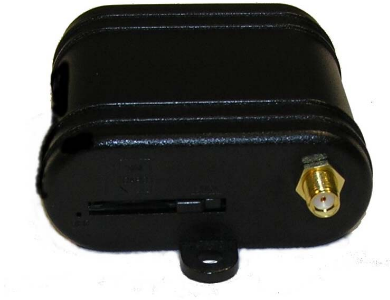
Figure 1 - Front view of GSM/GPRS SA-G+ modem.
