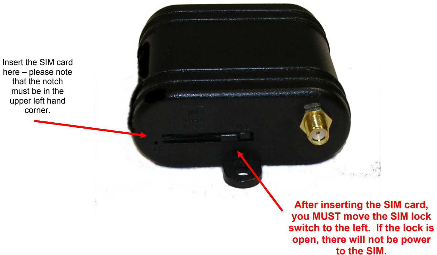
Figure 3 - Inserting a SIM Card in a GSM/GPRS SA-G+ Module
