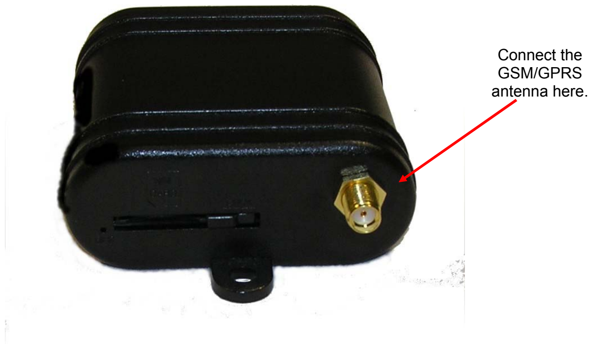
Figure 6 - GSM/GPRS SA-G+ Connecting the Antenna
